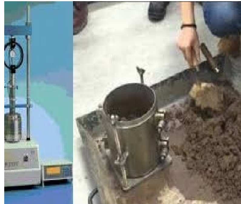
CBR SAMPLE PREPARATION
